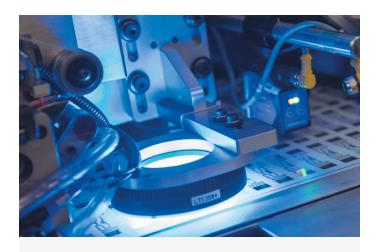
The communication capabilities of RFID tags must be tested intermittently during and/ or after packaging to ensure their integrity. Converters should partner with an experienced inlay manufacturer to anticipate and correct any production problems during the prototype and pilot production process. A knowledgeable partner can help to identify and correct any issues that could adversely impact the flexible circuitry inside the inlays.
