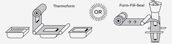
Flexible packaging material is unwound and formed into final package format Packages are formed on heat sealing or form-fill-seal equipment.
