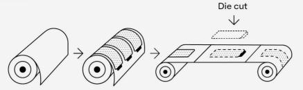
Label is printed and die cut, still on a roll with liner
