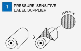
Pressure-sensitive material is created Adhesive is laminated onto film to create pressure-sensitive construction in roll form. 2 LABEL CONVERTER PRINTER AND DIECUTTER
